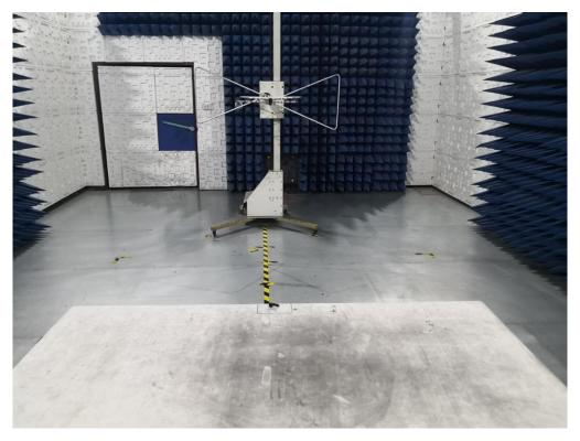
RADIATED EMISSION TEST SETUP ABOVE 1GHz
