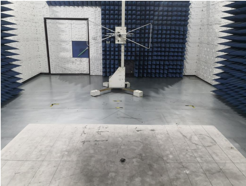
RADIATED EMISSION TEST SETUP ABOVE 1GHZ
