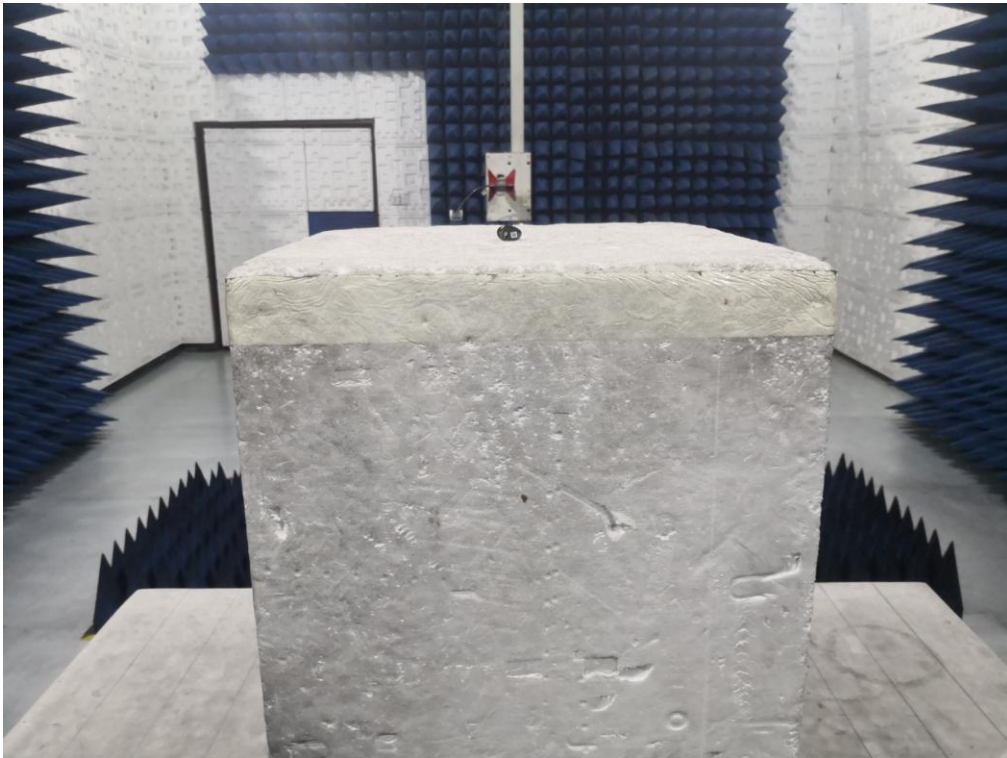
RADIATED EMISSION TEST SETUP ABOVE 1GHZ
