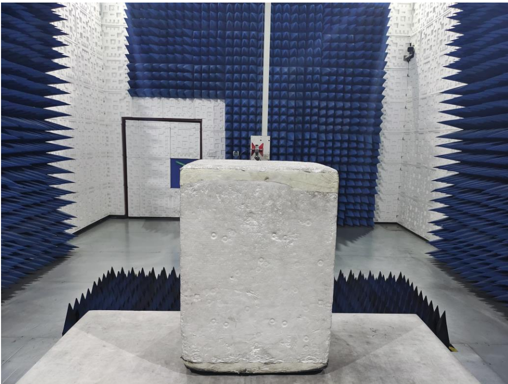
RADIATED EMISSION TEST SETUP ABOVE 1GHz
