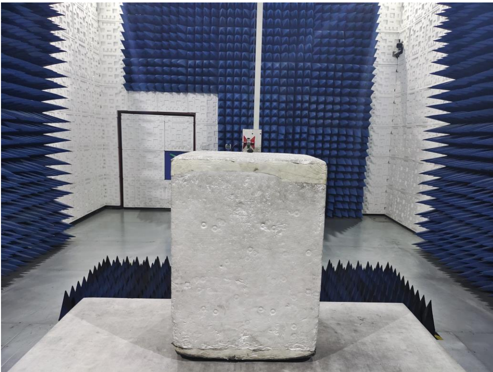
RADIATED EMISSION TEST SETUP ABOVE 1GHz
