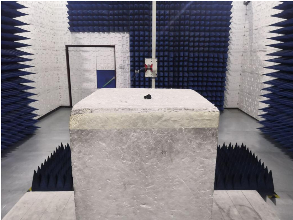
RADIATED EMISSION TEST SETUP ABOVE 1GHz
