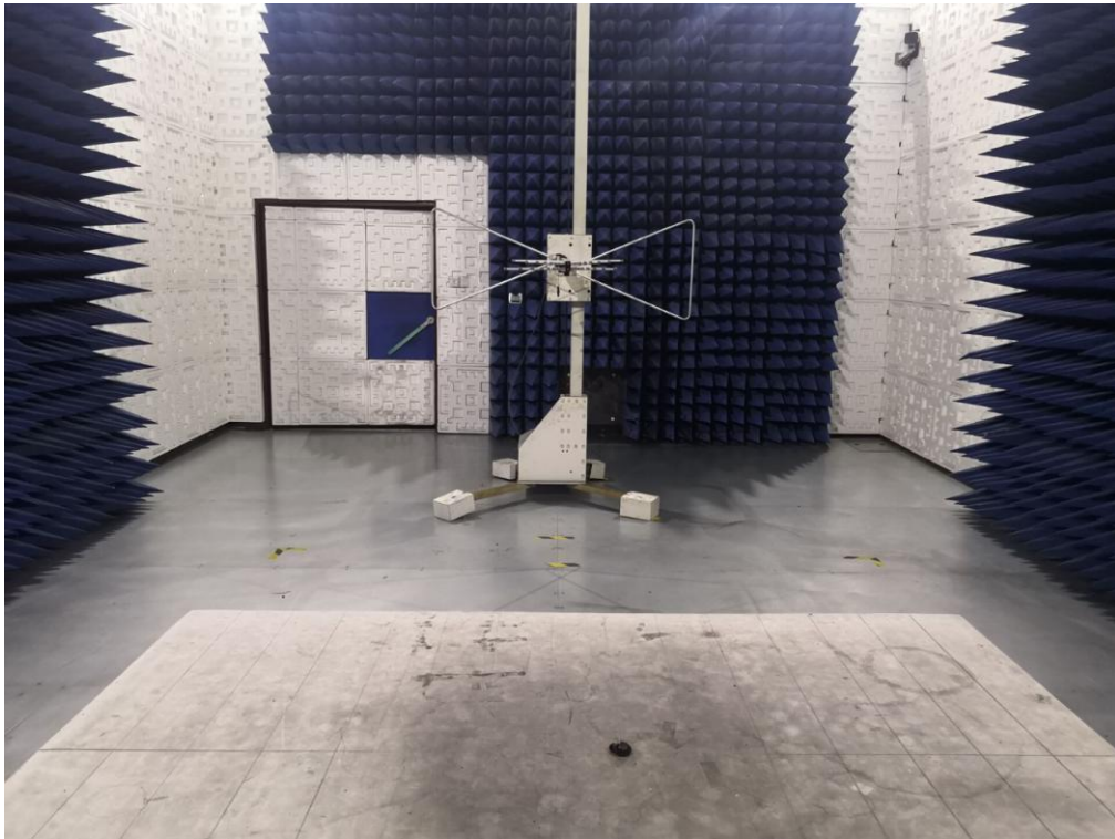
RADIATED EMISSION TEST SETUP ABOVE 1GHz
