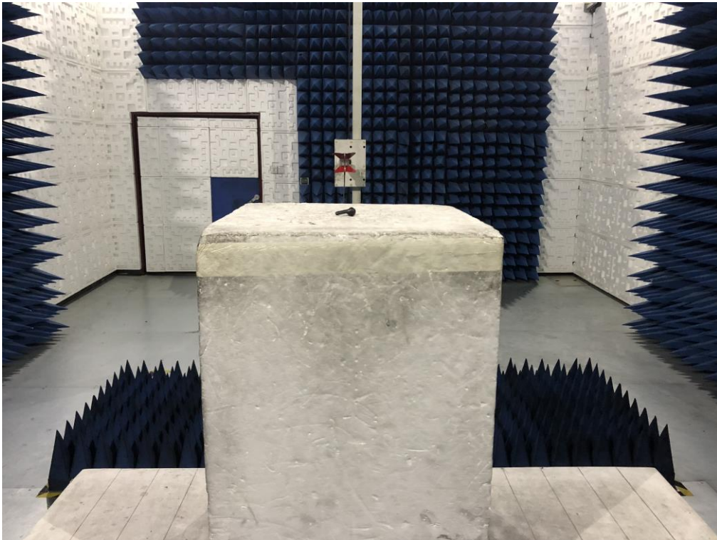
RADIATED EMISSION TEST SETUP ABOVE 1GHZ
