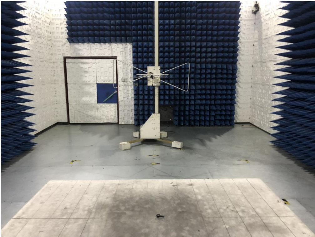
RADIATED EMISSION TEST SETUP ABOVE 1GHZ
