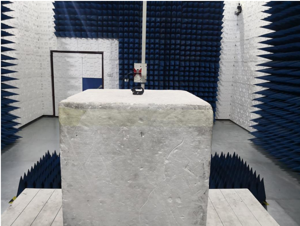
RADIATED EMISSION TEST SETUP ABOVE 1GHZ
