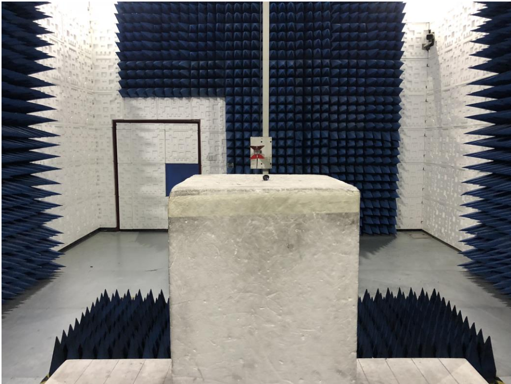
RADIATED EMISSION TEST SETUP ABOVE 1GHZ
