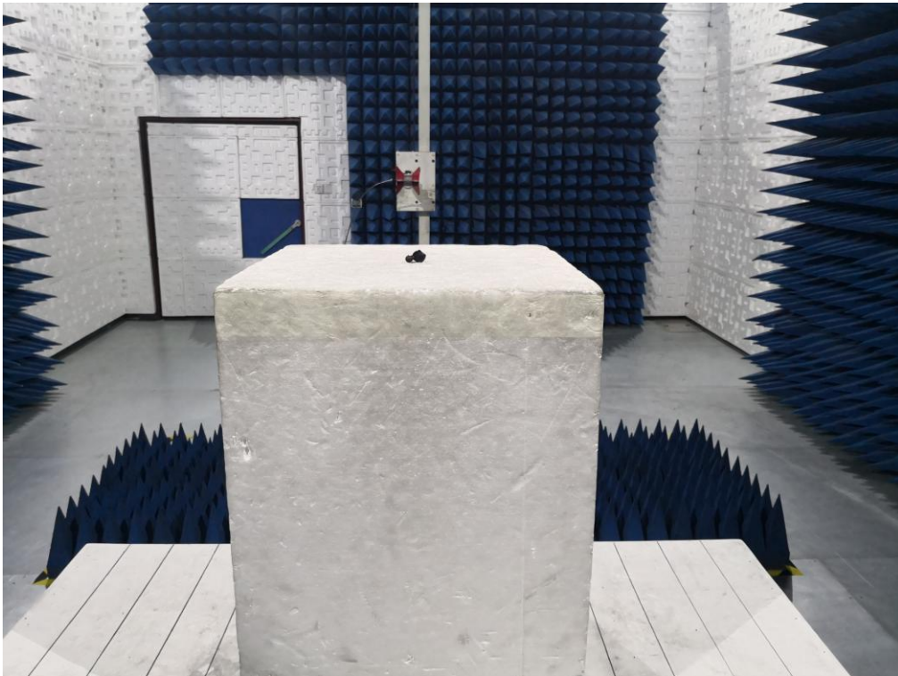
RADIATED EMISSION TEST SETUP ABOVE 1GHZ
