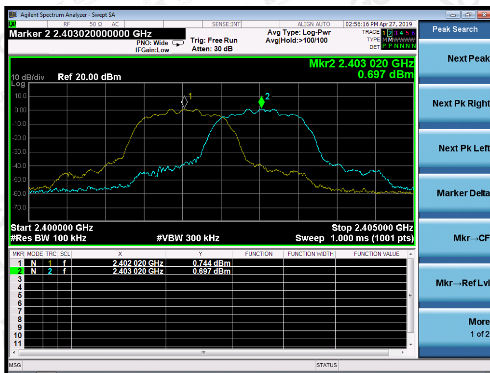
TEST PLOT FOR FREQUENCY SEPARATION
