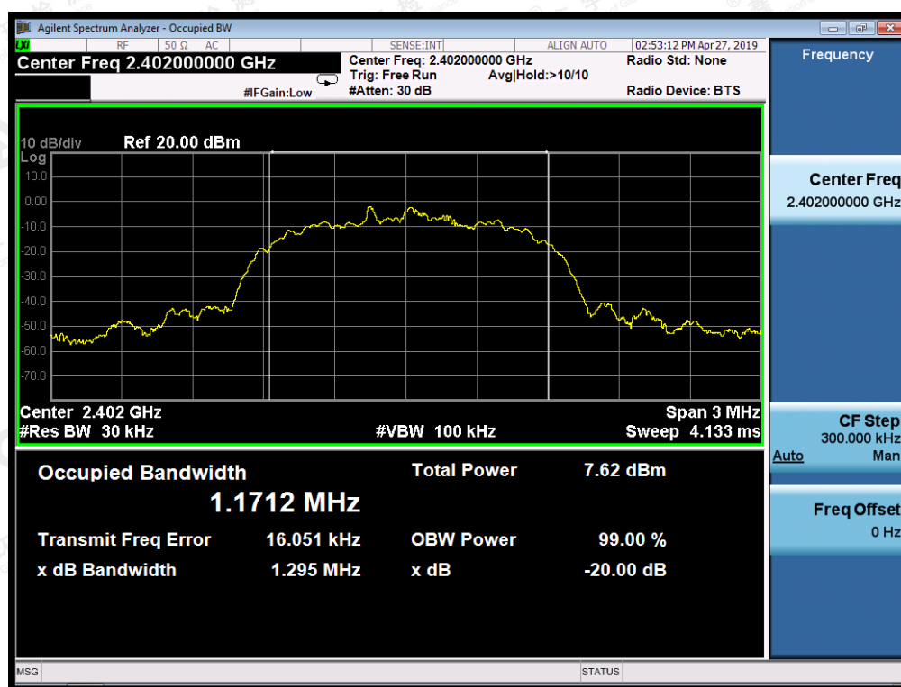
TEST PLOT OF BANDWIDTH FOR LOW CHANNEL
