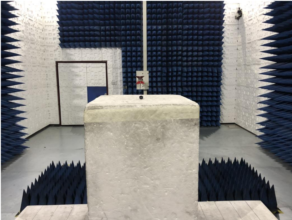
RADIATED EMISSION TEST SETUP ABOVE 1GHZ
