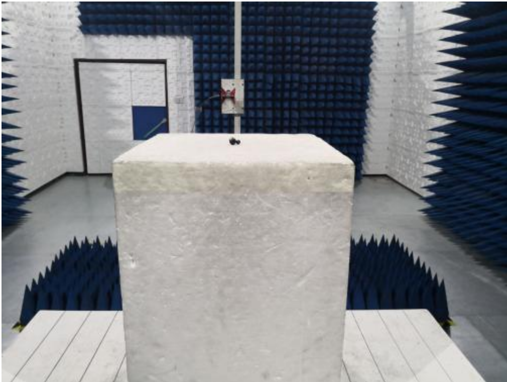
RADIATED EMISSION TEST SETUP ABOVE 1GHZ
