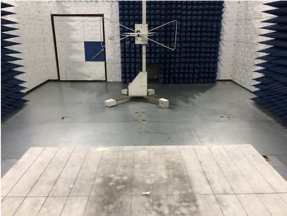
RADIATED EMISSION TEST SETUP ABOVE 1GHZ
