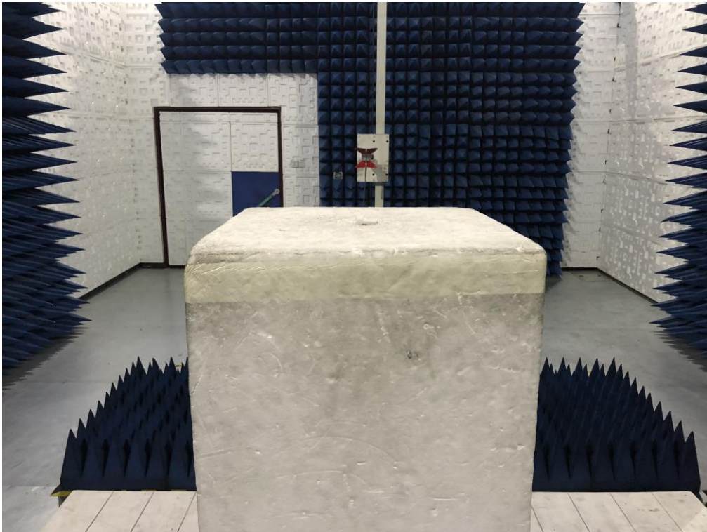
RADIATED EMISSION TEST SETUP ABOVE 1GHZ
