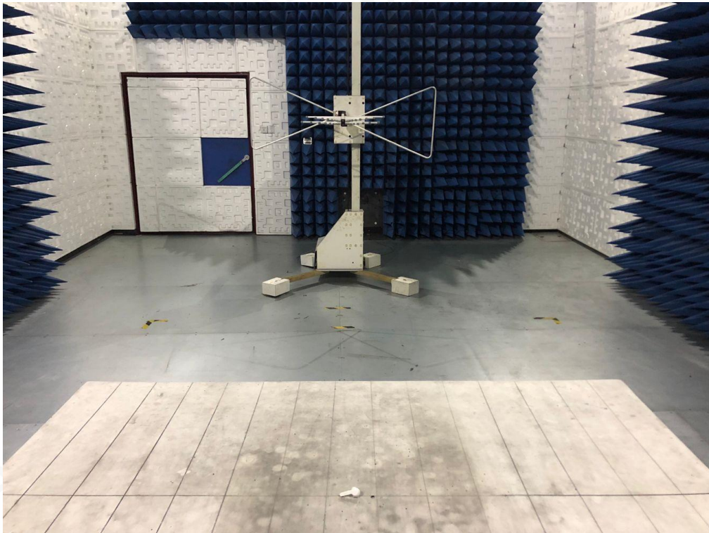
RADIATED EMISSION TEST SETUP ABOVE 1GHZ
