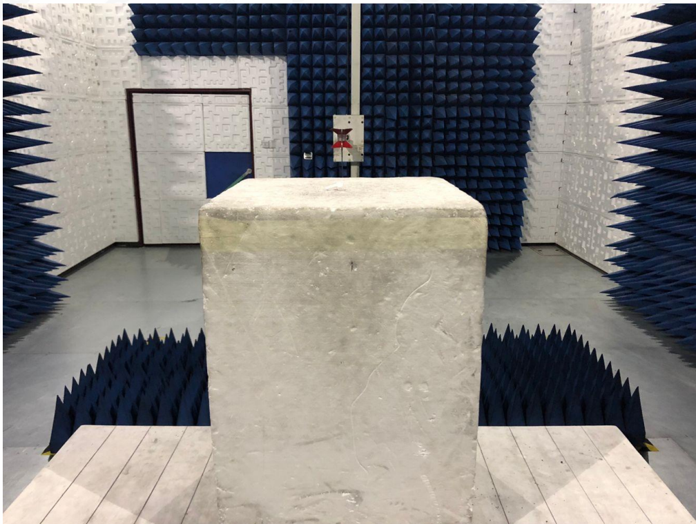
RADIATED EMISSION TEST SETUP ABOVE 1GHZ
