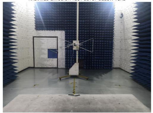
RADIATED EMISSION TEST SETUP ABOVE 1GHz
