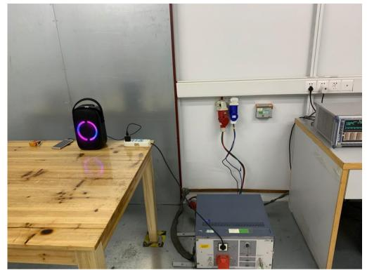
CONDUCTED TEST SETUP
