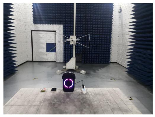
RADIATED EMISSION TEST SETUP ABOVE 1GHZ
