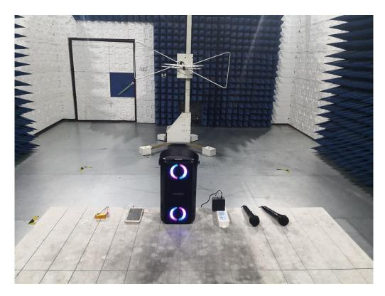
RADIATED EMISSION TEST SETUP ABOVE 1GHZ
