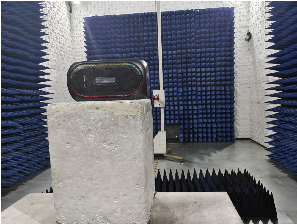
dRADIATED EMISSION TEST SETUP ABOVE 1GHz
