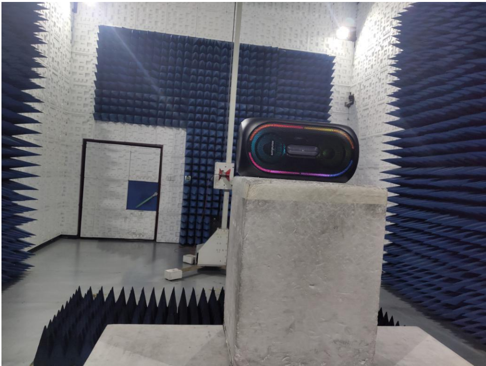
dRADIATED EMISSION TEST SETUP ABOVE 1GHz
