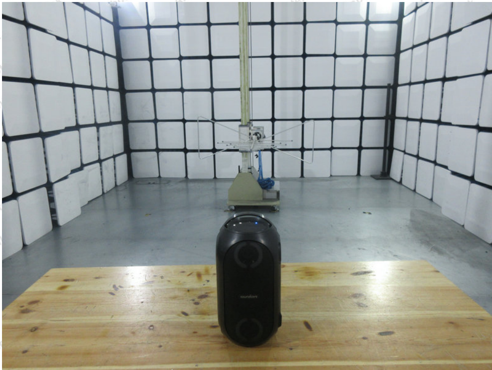
Photo of Radiation Emission Test
