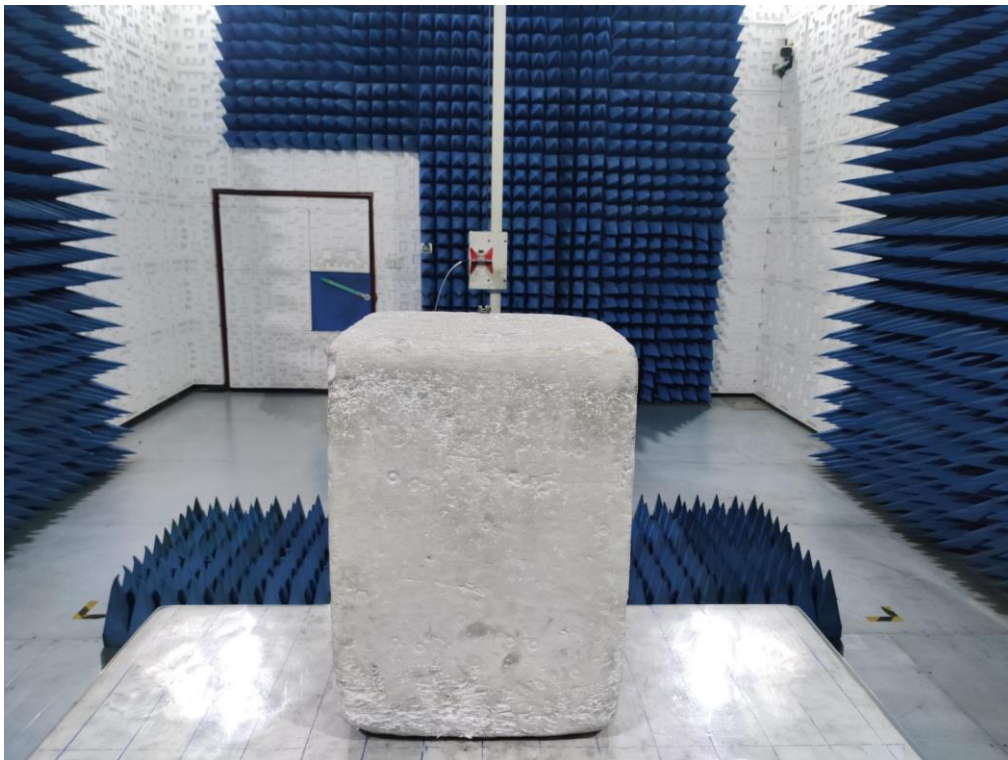
RADIATED EMISSION TEST SETUP ABOVE 1GHz
