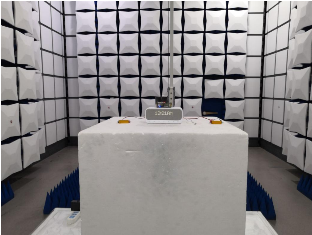
RADIATED EMISSION TEST SETUP ABOVE 1GHZ
