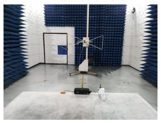
RADIATED EMISSION TEST SETUP ABOVE 1GHz
