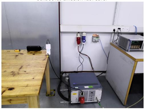
CONDUCTED TEST SETUP
