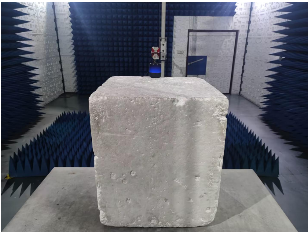
RADIATED EMISSION TEST SETUP ABOVE 1GHz
