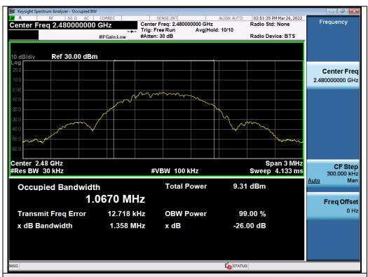
Test\_Graph\_LE1M\_ANT1\_2480\_1Mbps\_OBW Test Graphs of DTS Bandwidth
