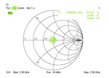
Calibrated return loss: -29.54dB; Measurement return loss: -29.55dB(within 20%)
