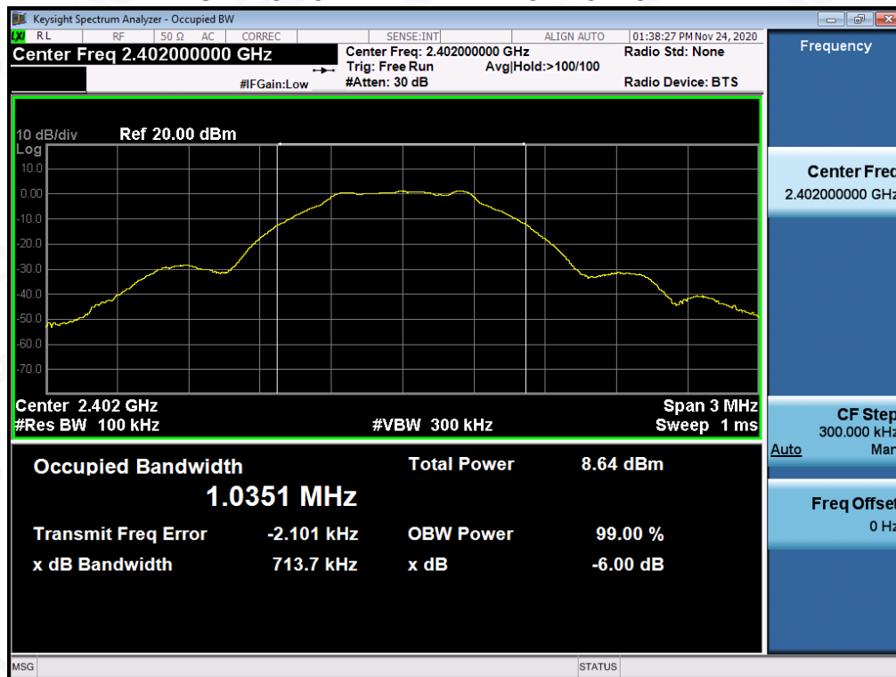
TEST PLOT OF BANDWIDTH FOR LOW CHANNEL
