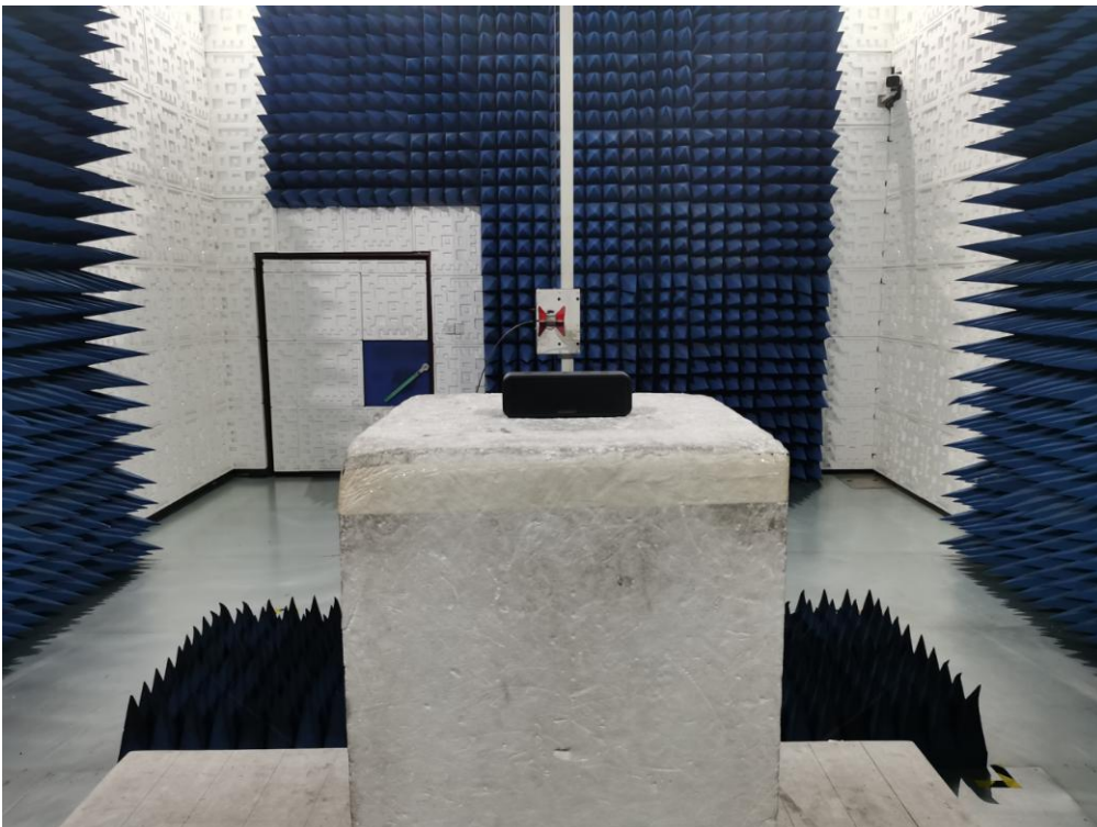
RADIATED EMISSION TEST SETUP ABOVE 1GHz
