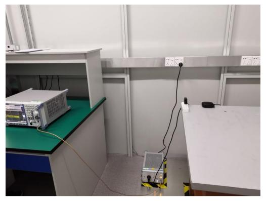
RADIATED EMISSION TEST SETUP
