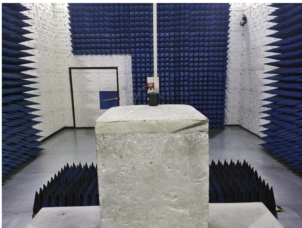
RADIATED EMISSION TEST SETUP ABOVE 1GHz
