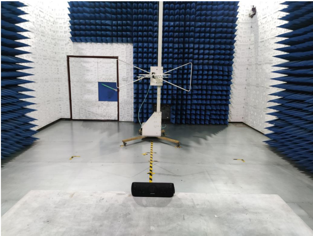
RADIATED EMISSION TEST SETUP ABOVE 1GHz
