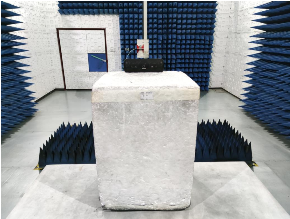
RADIATED EMISSION TEST SETUP ABOVE 1GHz
