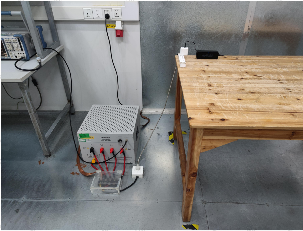
Photo of Conducted Emission Measurement
