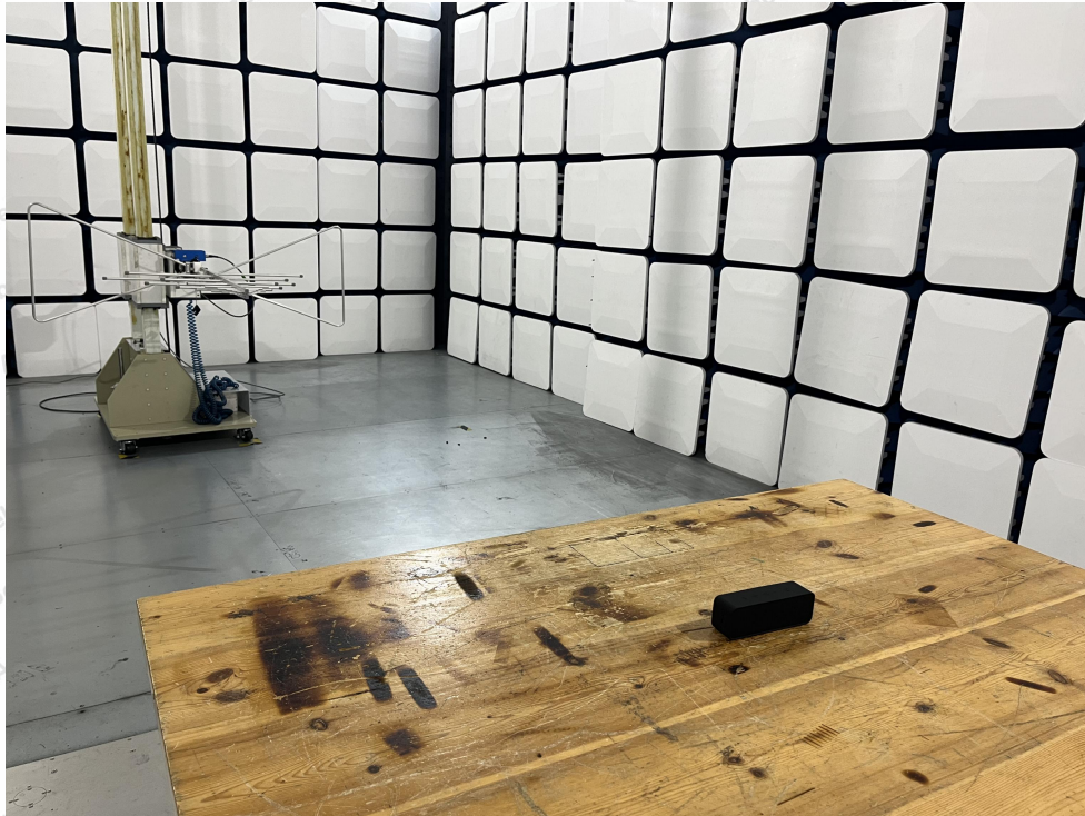
Photo of Radiation Emission Test
