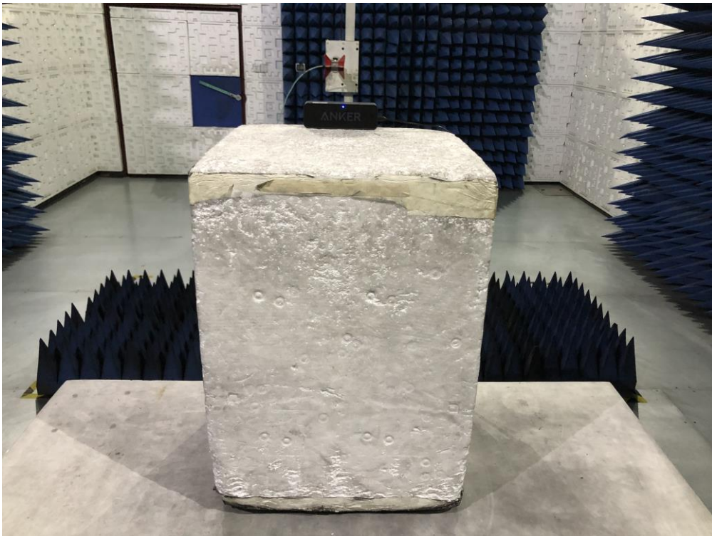
RADIATED EMISSION TEST SETUP ABOVE 1GHz
