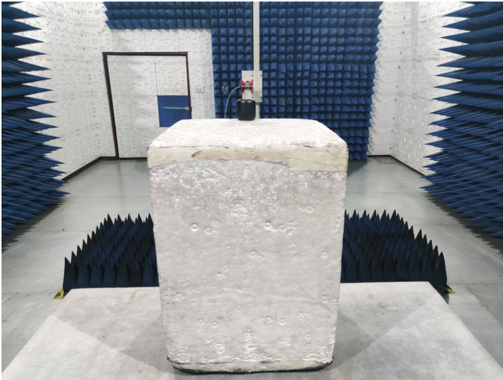
RADIATED EMISSION TEST SETUP ABOVE 1GHz
