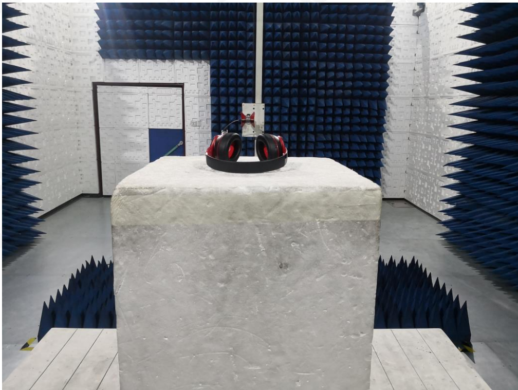
RADIATED EMISSION TEST SETUP ABOVE 1GHZ
