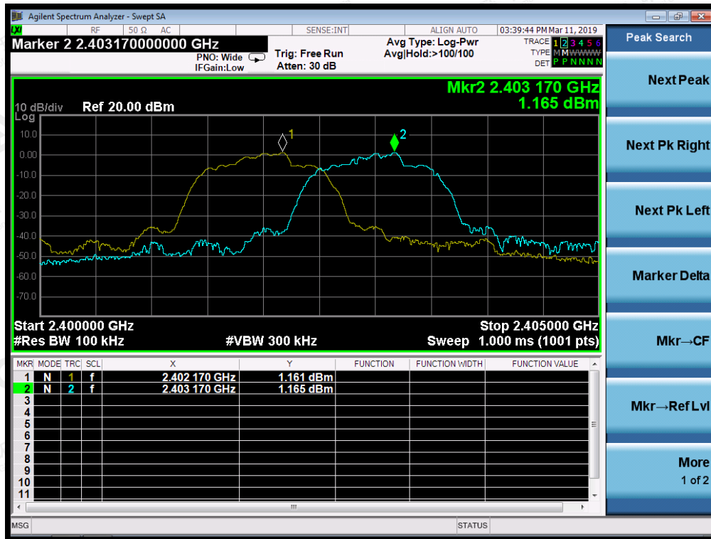
TEST PLOT FOR FREQUENCY SEPARATION ( 1Mbps )
