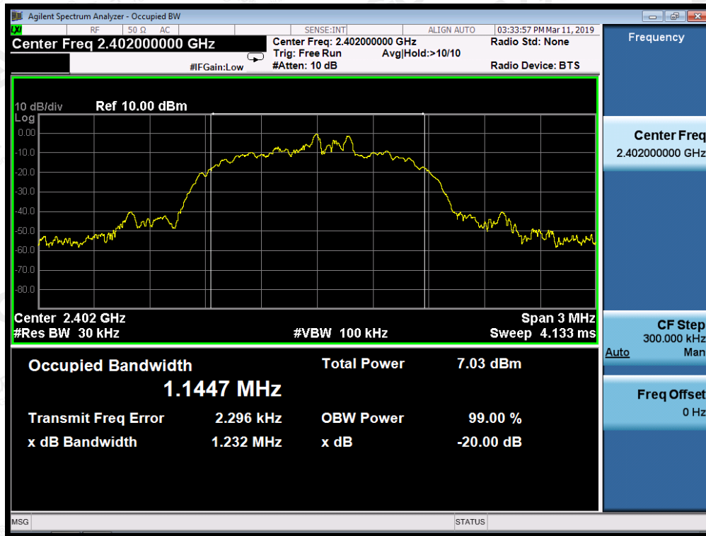
TEST PLOT OF BANDWIDTH FOR LOW CHANNEL
