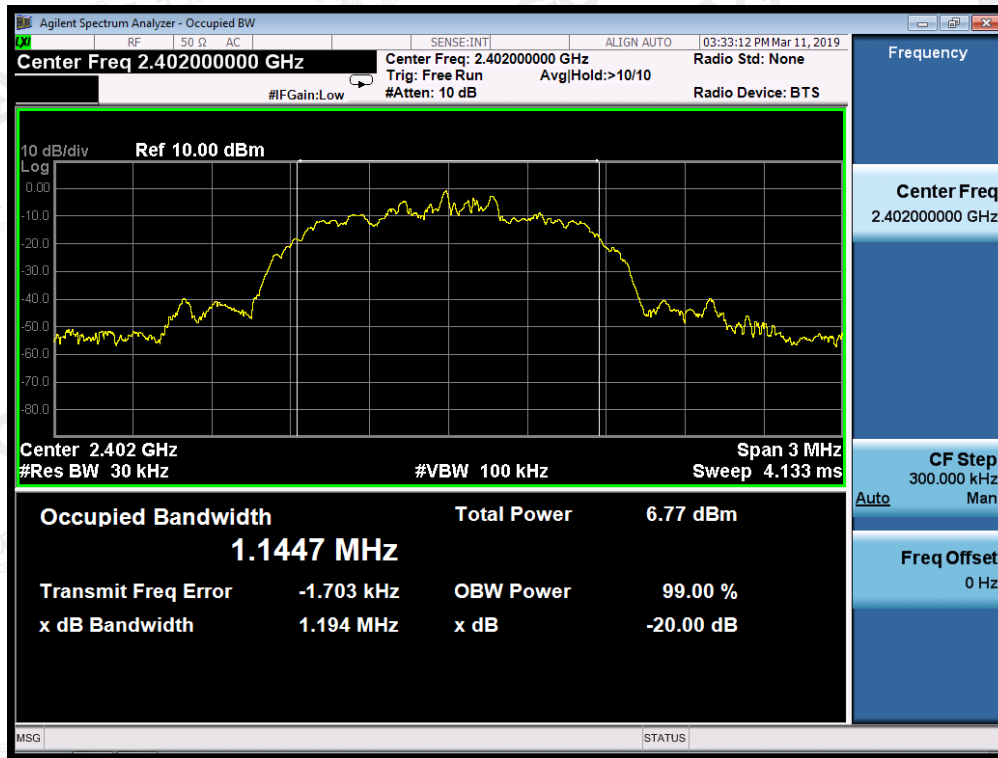
TEST PLOT OF BANDWIDTH FOR LOW CHANNEL
