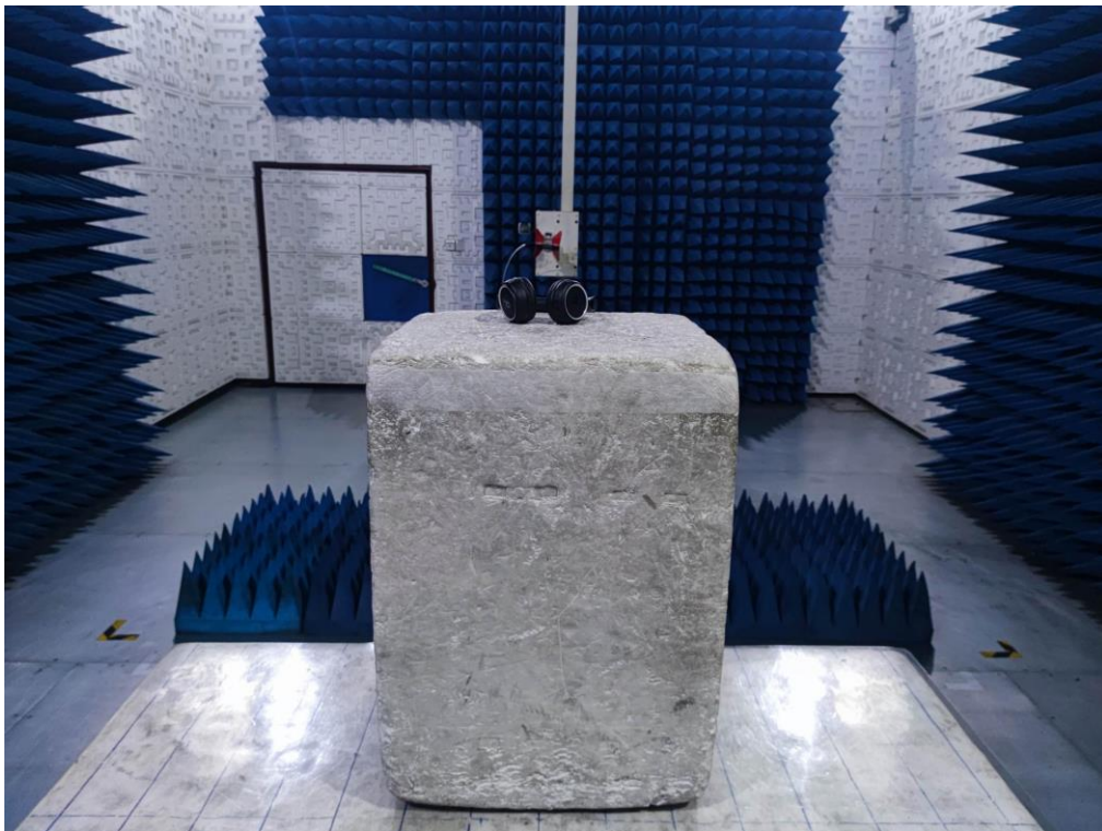
RADIATED EMISSION TEST SETUP ABOVE 1GHz
