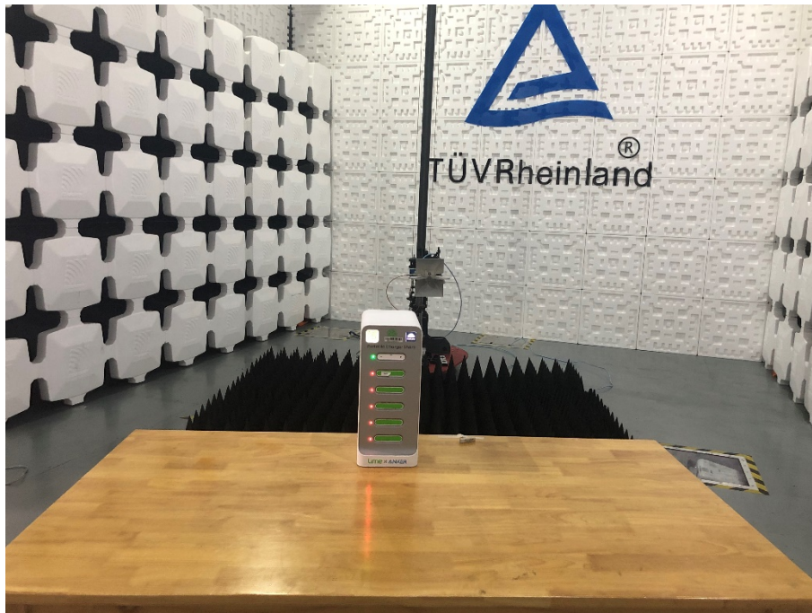
Photograph 5: Set-up for Radiated Emission, above 1GHz
