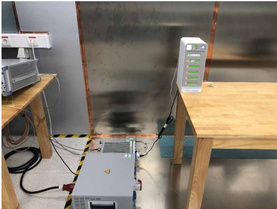
Photograph 3: Set-up for Conducted Emission on AC Mains
