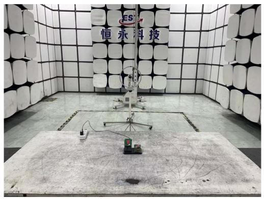
Radiated Test (30MHz-1GHz)
