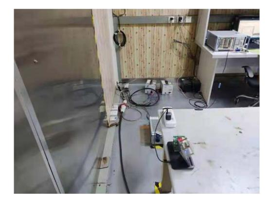
Radiated Test (9kHz-30 MHz)
