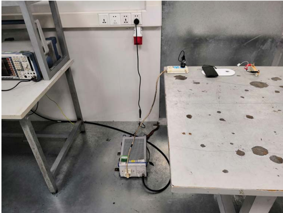
Photo of Conducted Emission Measurement
