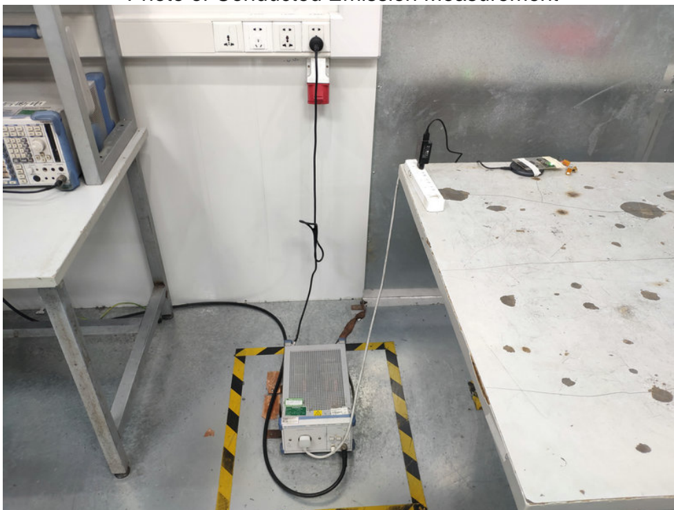
FCC ID: 2AOKB-A2509 Photo of Conducted Emission Measurement
