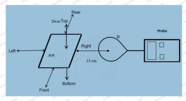
Note: Measurements should be made at 15 cm surrounding the EUT and 20cm above the top surface of the EUT.
