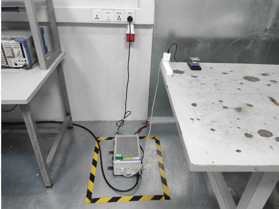
Photo of Conducted Emission Measurement
