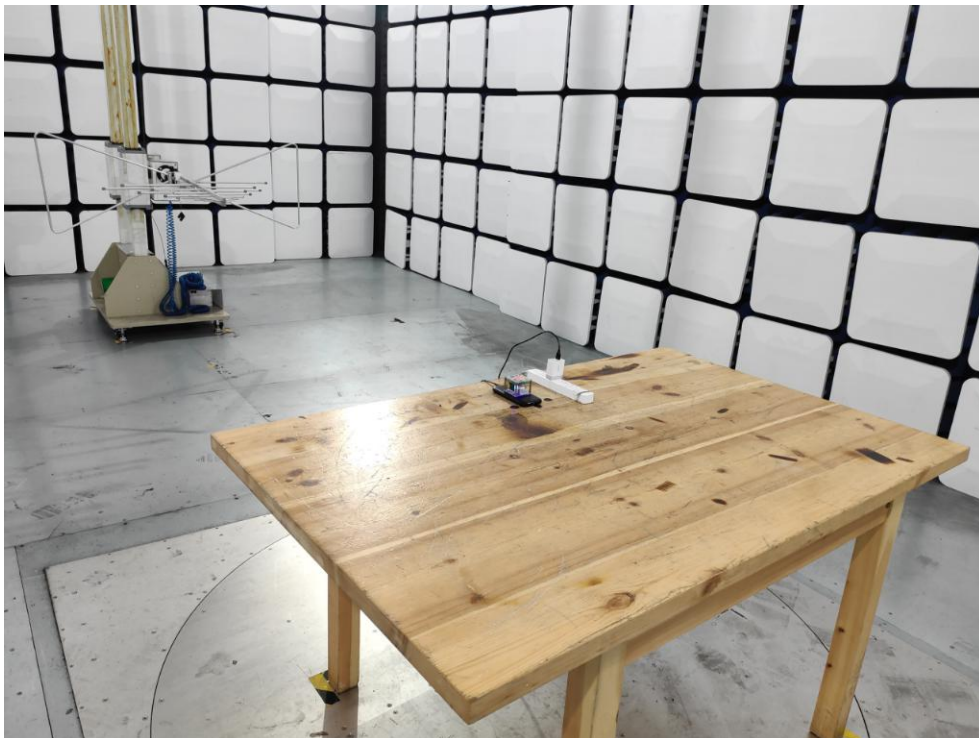
Photo of Radiation Emission Test
