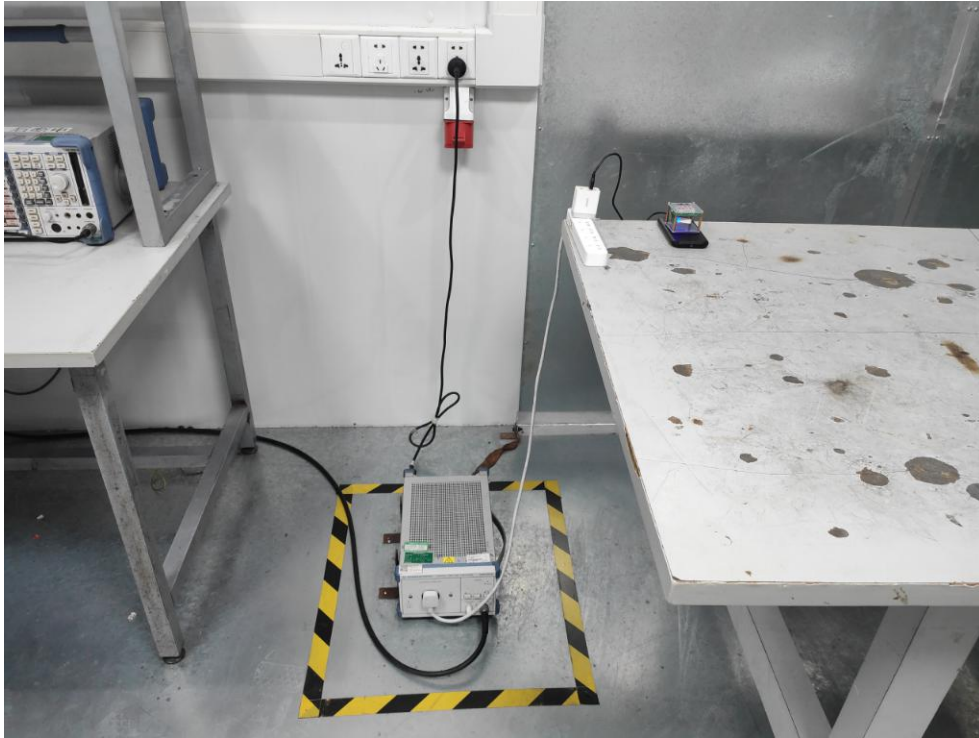
Photo of Conducted Emission Measurement
