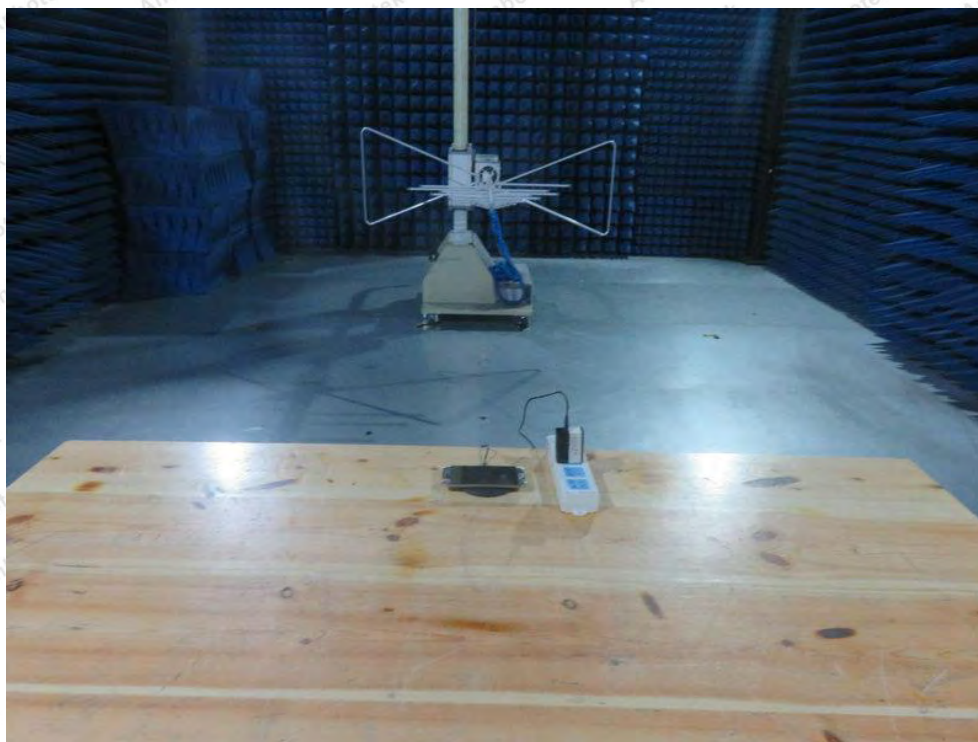
Photo of Radiation Emission Test
