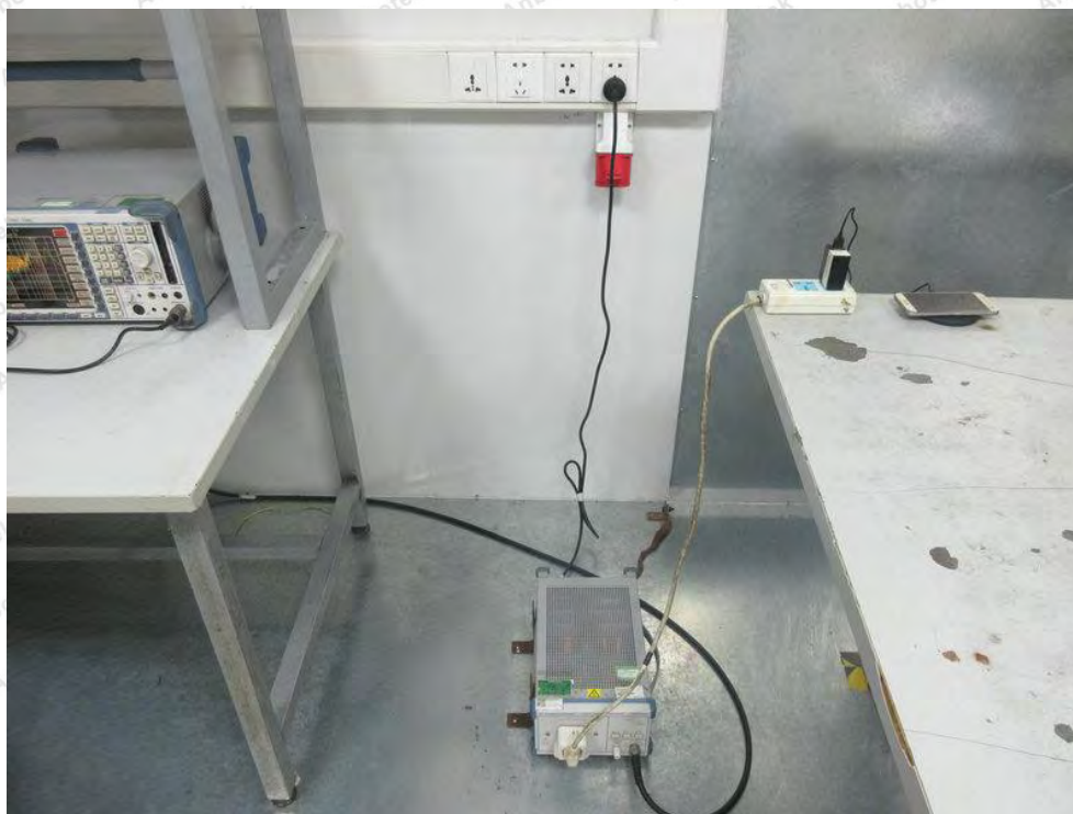
Photo of Conducted Emission Measurement
