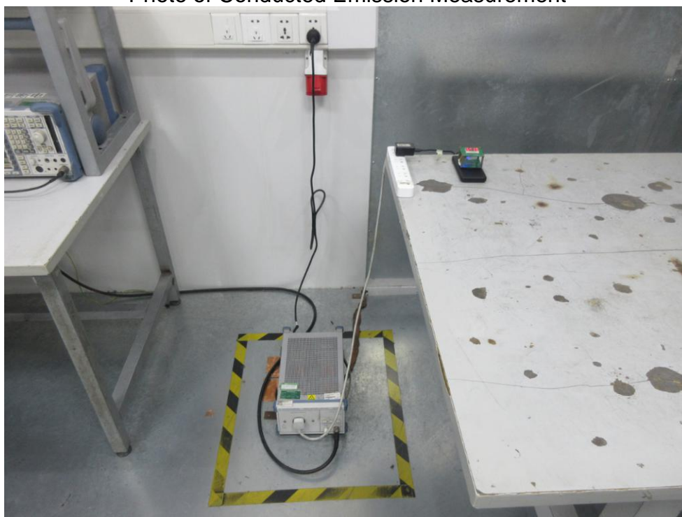
FCC ID: 2AOKB-A1615 Photo of Conducted Emission Measurement
