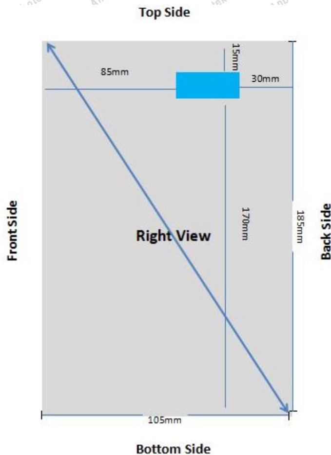
Positions for SAR tests; Body mode
