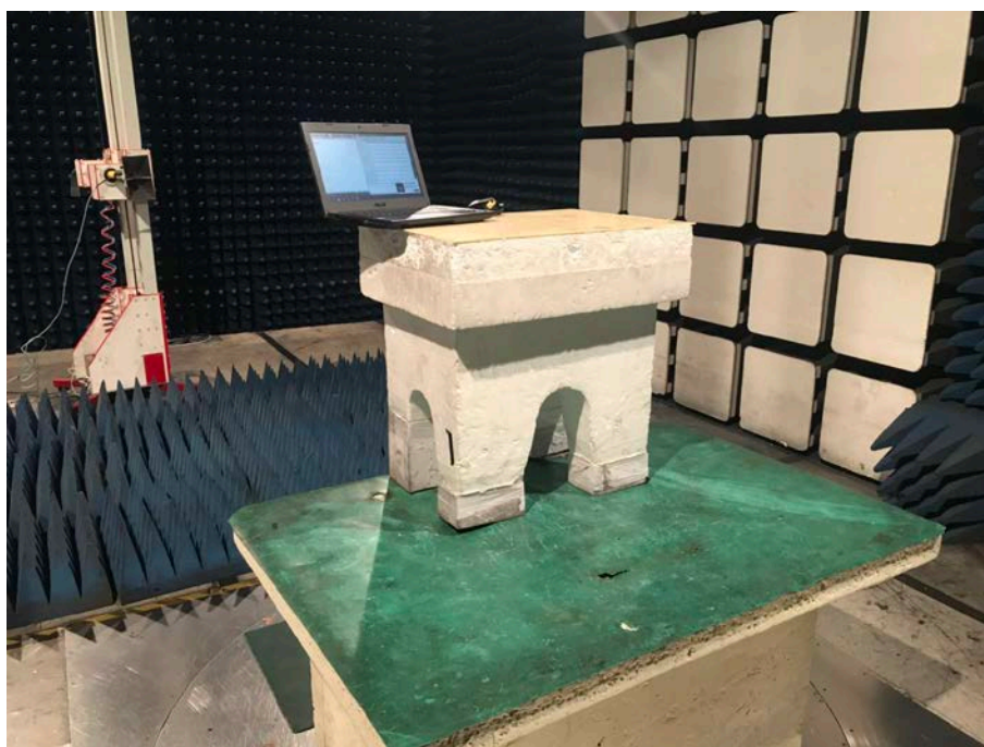
Spurious Emission Test Setup (Above 1GHz)
