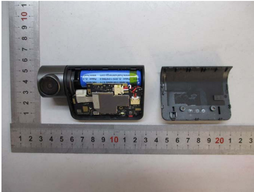
EUT – Cover off View-2
