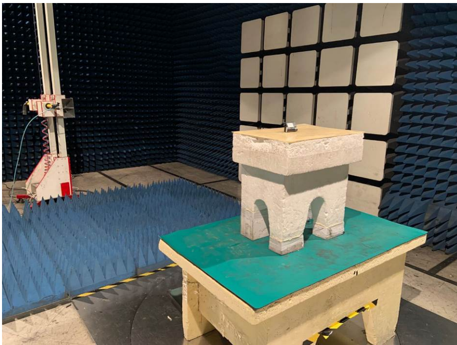
Spurious Emission Test Setup (Above 1GHz)
